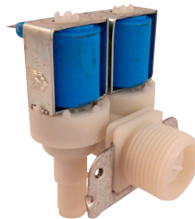
Clave. PRI340020035 Valve, Water, 2-Way, 220-240V/50-60Hz, 3/4G Inlet, 14.5mm Outlets (2), With 14 L/Min Flow Restrictor, Alliance.
